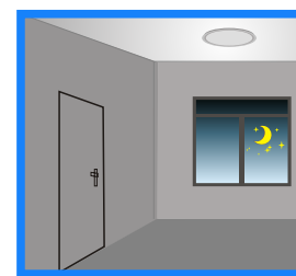
After stand-by period, the sensor switches off the lamp if no motion is detected in its detection zone.
